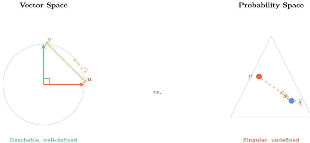
Figure 4: The fundamental asymmetry between vector geometry and probability geometry. Left: Orthogonal vectors have a well-defined Euclidean distance ( \sqrt{2} on the unit circle). Right: Distributions with disjoint support (the probabilistic analog of orthogonality) have D_{\text{KL}} = +\infty . The geometric framework handles independence naturally; the information-theoretic framework breaks at the same point.
