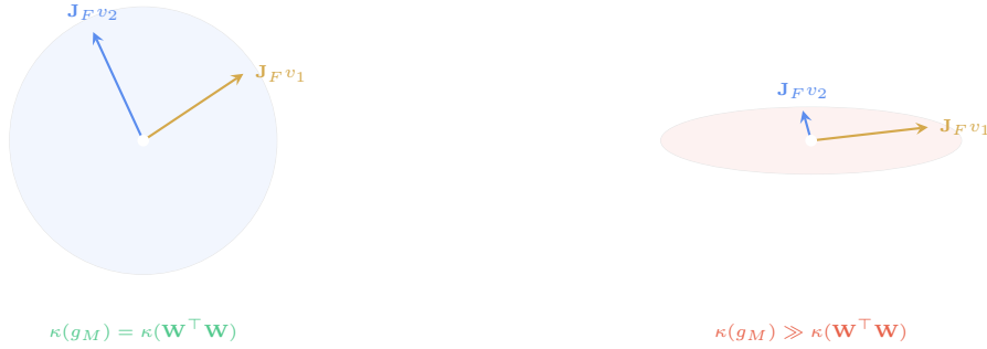
Figure 3: The pullback metric as an ellipsoid of tangent vector lengths. Left: Linear activation preserves the conditioning of \mathbf{W} . Right: Sigmoid saturation compresses one axis dramatically, worsening the condition number and distorting distances.
