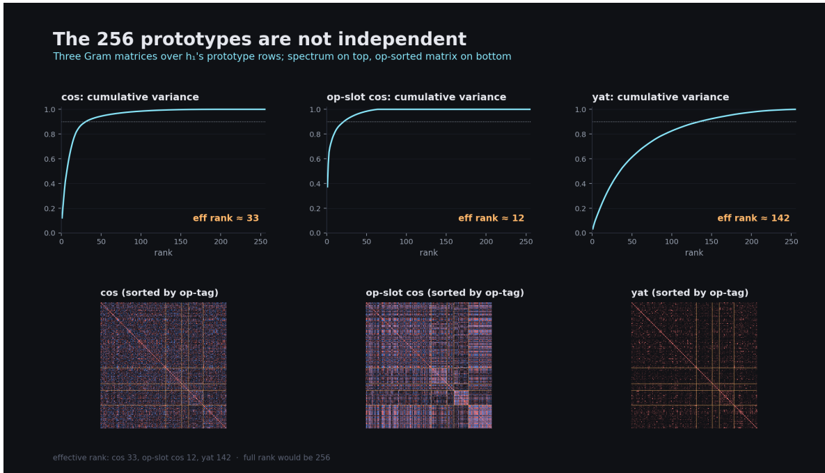
Figure 12: Three Gram matrices over h_1 's 256 prototype rows. Top: cumulative variance captured by the sorted spectrum (cosine, op-slot-only cosine, and the \bar{Y}at function itself). Bottom: the corresponding Gram matrices permuted by operator-tag. eff-rank annotations are on each top panel. The op-slot eff-rank \approx 12 means h_1 effectively allocates roughly one dozen distinct operator-conditioned prototype shapes, replicated across the trunk in varying magnitudes.
